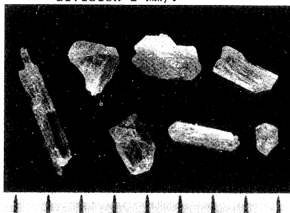
Fig.5. Grown \text{NaGdSiO}_4 crystals (1 division=1 mm).
